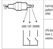
Each Up / Down pin is pulled to 3.3 V with CPU GPIO.
