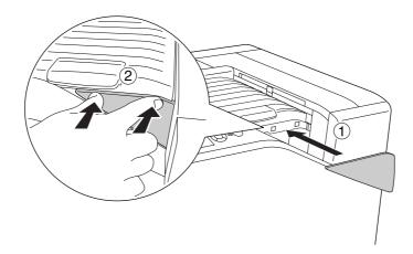
16. Remove the cover on the printer.
