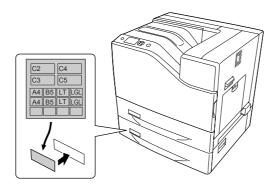
10. Load a stack of the desired paper with the printable surface facing up.
