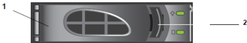
Figure 18. Disk tray handle and release latch
