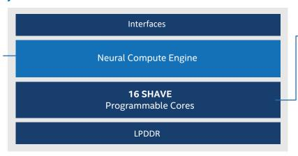
VLIW (DSP) programmable processors are optimized for complex visions and imaging workloads
