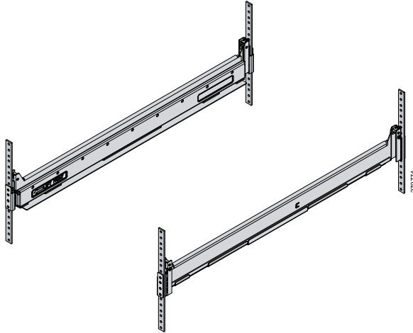
Figure 28: Round Hole Adapter and Rails Installed in a Rack
