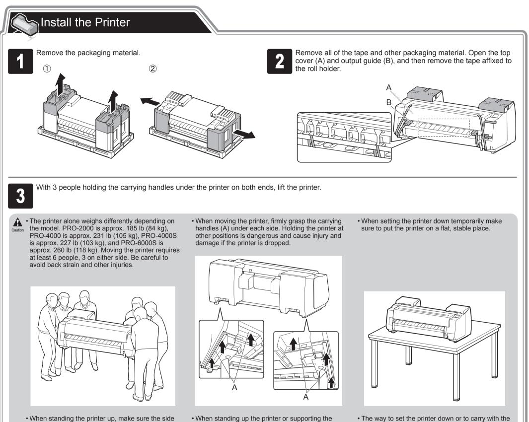
• When standing the printer up, make sure the side with the control panel is up, and place cardboard or other material underneath to prevent scratching. Furthermore, make sure that the weight of the printer is taken by the corner of the printer. If the weight is taken by any other part of the printer, the printer may become damaged.
