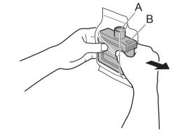
• Never touch the ink holes (A) 0 or metal contacts (B). Touching mportant these parts may cause stains, damage the ink tank, and affect print quality.
