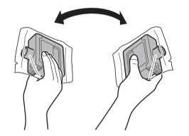
• Failure to shake the ink tanks may result 0 in reduced print quality because ink nportant ingredients have settled on the bottom of the tank.
