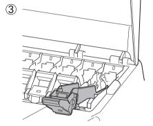
• Make sure the ink tank lock lever stays in the locked position. 0
