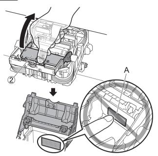
(1) Remove the print head from the box and bag, and peel off the fixing tape. 2) Grasp the blue handle and remove the print head.
