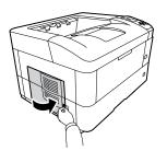
Wipe the vent holes on the right side of the printer with a soft, dry cloth to remove dust and dirt.
