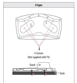
Screw: M5 x L (\*L: Table depth + 8~10 mm)
