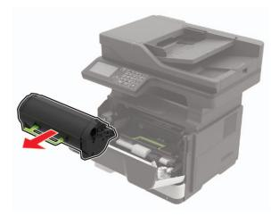
**3** Remove the used imaging unit.
